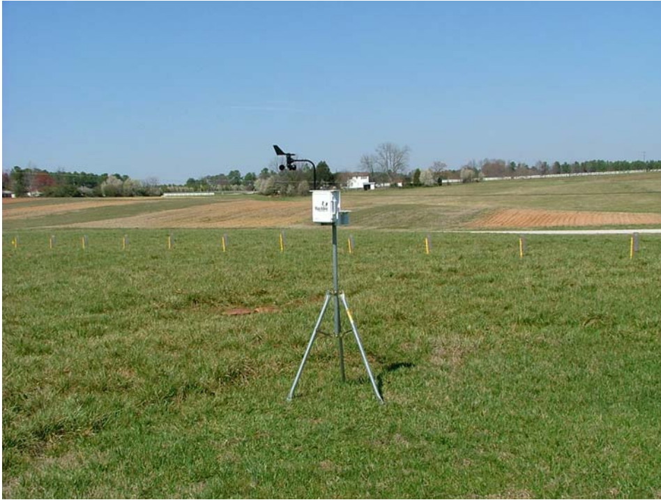
Figure 3. Watchdog weather station used to collect wind speed and direction data. Collection gages in background.
