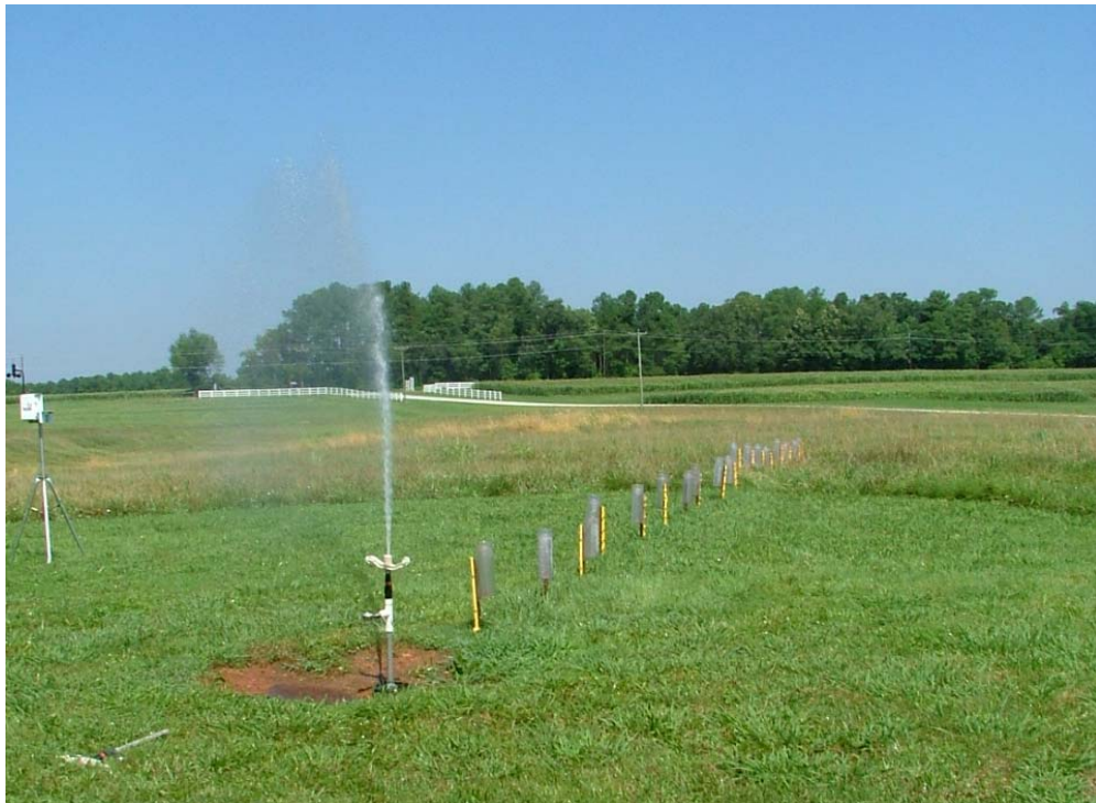
Figure 2. Field trials at LWFL. Profile data for a Senninger stationary system is being collected in this photo.
